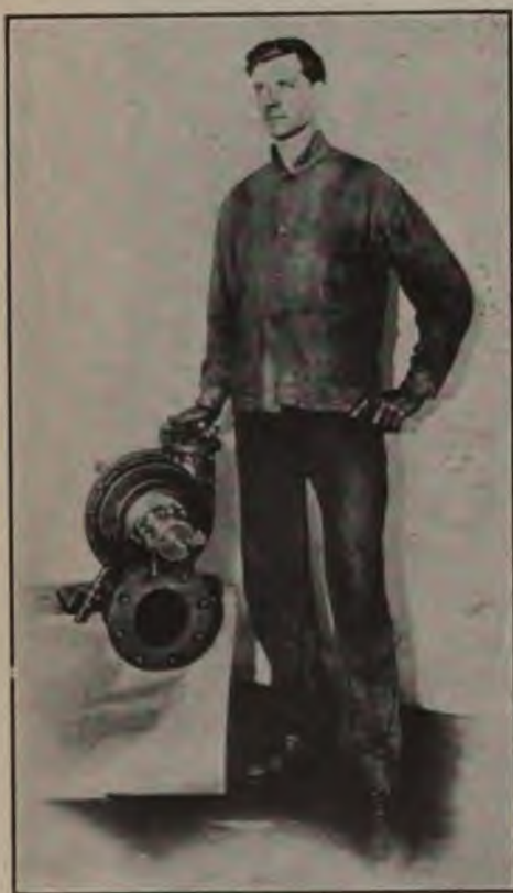
THIS ABSURDLY SMALL ENGINE — TESLA'S SMALLEST MODEL — DEVELOPS 110 HORSE POWER
