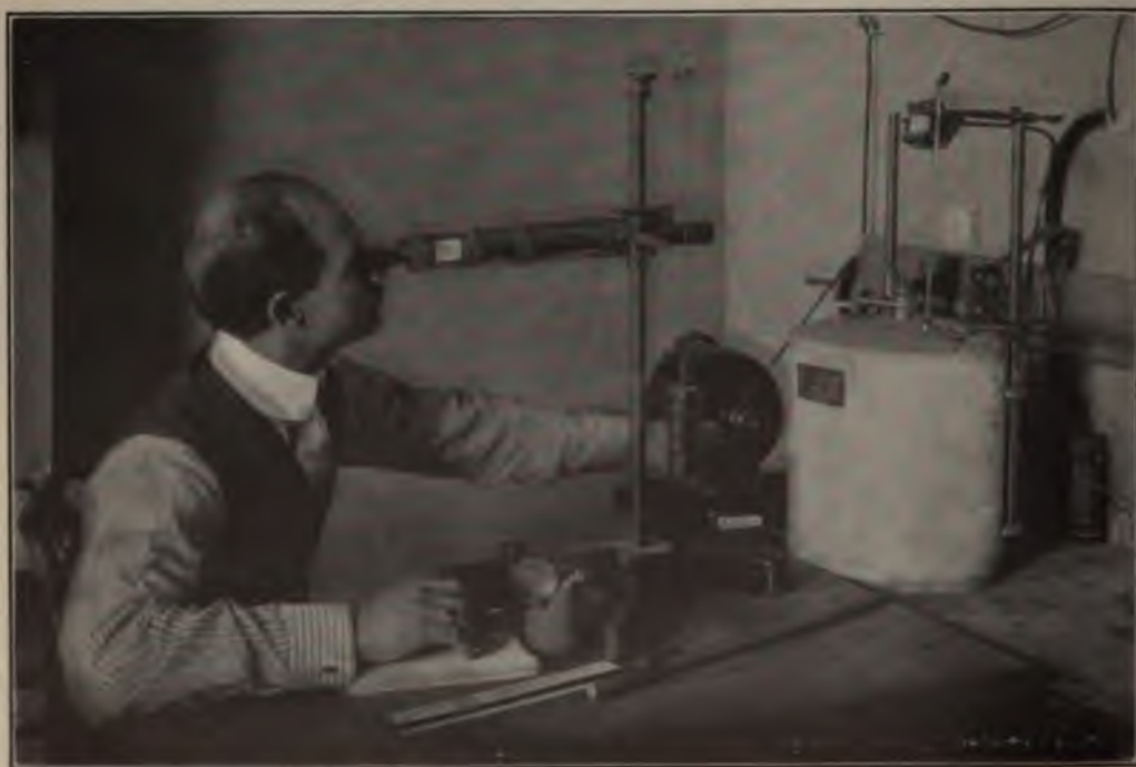
WATCHING THE THERMOMETER THROUGH A MAGNIFYING GLASS TO GET THE EXACT TEMPERATURE BY WHICH TO TELL THE NUMBER OF HEAT UNITS IN THE PIECE OF COAL IN THE CALORIMETER. MORE THAN $4,000,000 WORTH OF COAL IS BOUGHT FOR THE GOVERNMENT EVERY YEAR IN ACCORDANCE WITH THE BUREAU'S TESTS
