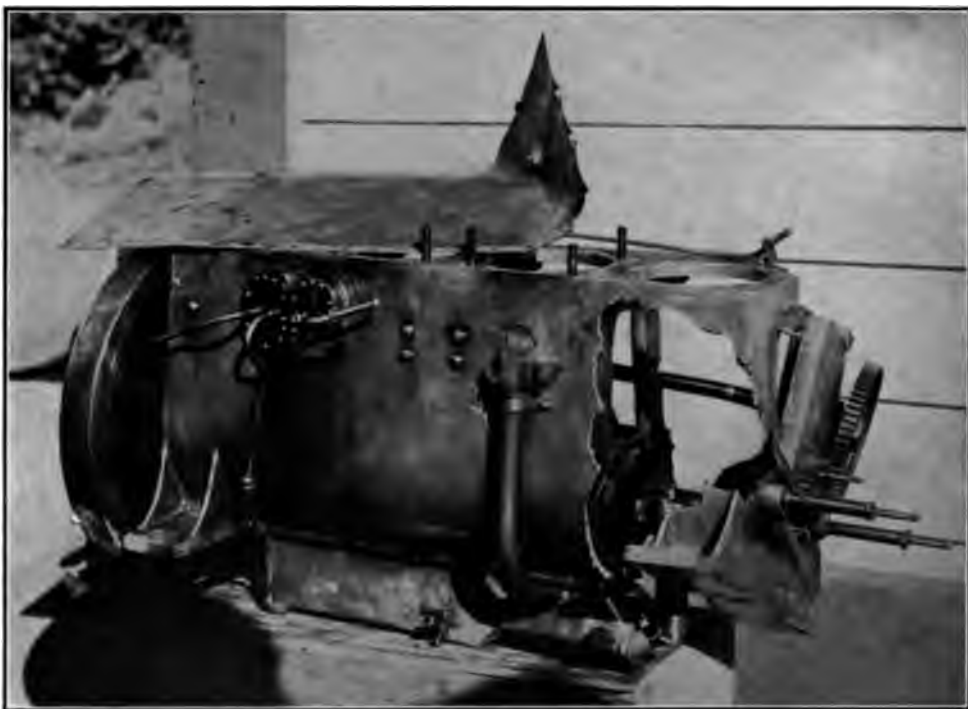
A CYLINDER THAT BLEW OUT 4,000 FEET IN THE AIR WRECKING THE ENGINE AND FILLING RODGERS'S ARM WITH FLYING PIECES OF STEEL, IN SPITE OF WHICH, HOWEVER, HE MADE THE THREE QUARTERS OF A MILE DESCENT IN SAFETY
