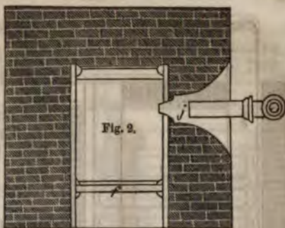
Fig. 2 is a horizontal section of the same on the level of the tuyere.
