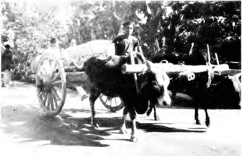
2. Bamboo provides the yoke and the "bed" for ox carts, the principal means of transporting building materials in India, Pakistan, and many other parts of the Far East.
