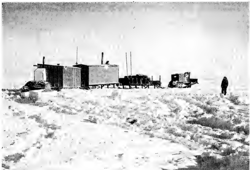
2. A "cat-train" bound for survey operations near Point Barrow. Long hitches of sleds and "wainigans" carry the surveyors, their instruments, and their habitation as a relatively self-sustained unit.
