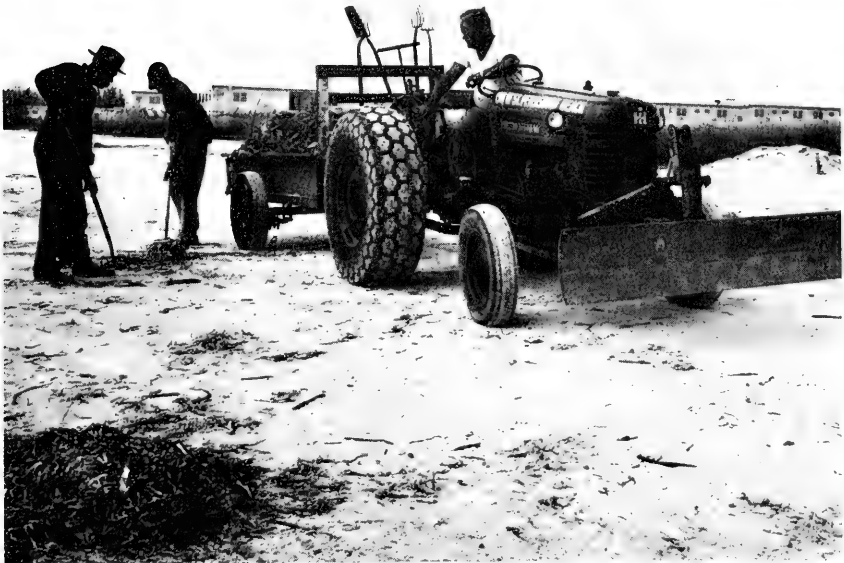
2. Cleanup equipment used at City of St. Petersburg Beach. Blade piles decaying fish and seaweed, and pitchforks are used to load beach debris into trailers. (Photograph courtesy of St. Petersburg Times .)
