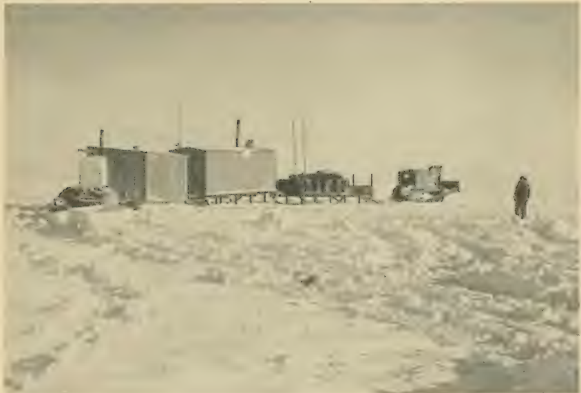
2. A "cat-train" bound for survey operations near Point Barrow. Long hitches of sleds and "wanigans" carry the surveyors, their instruments, and their habitation as a relatively self-sustained unit.
