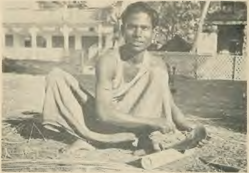
1. As demonstrated by this bamboo worker at Chittagong, East Pakistan, who is making lashings to take the place of nails, no complicated or costly machinery is required to process bamboo for building purposes.
