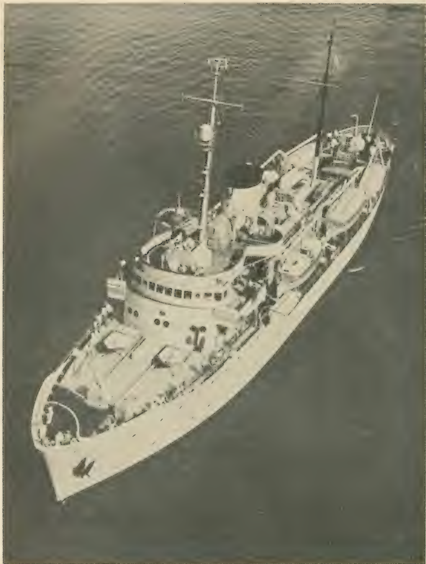
The Explorer , one of the four modern survey ships now in use, was built in 1940 for Alaskan Survey work. She displaces 1,900 tons and has a cruising radius of 6,000 miles at 15 knots.
