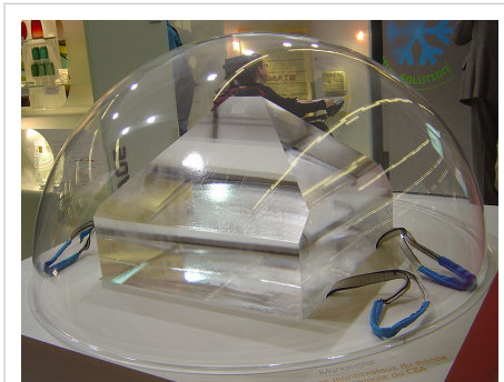
A large monocrystal of potassium dihydrogen phosphate grown from solution by Saint-Gobain for the megajoule laser of CEA.
