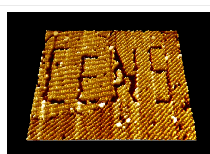
Nanomanipulation via STM of a self-assembled organic semiconductor monolayer (here: PTCDA molecules) on graphite, in which the logo of the Center for NanoScience (CeNS), LMU has been written.
