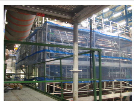
September 2005: the main barrel section of the ATLAS hadronic calorimeter, waiting to be moved inside the toroid magnets.
